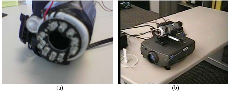
Figure 3. The left picture shows our camera detector unit. We outfitted a Sony HandyCam, placed in NightShot mode, with a collection of IR transmitters and covered the lens with a narrow bandpass IR filter. The right picture shows our camera detector coupled with a projector to neutralize cameras in the environment.
