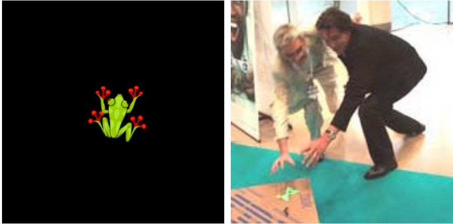
Figure 2. (left) Image of a frog (part of an animation sequence) with black background. (right) Jumping Frog , a game-like application where participants chase an animated-projected frog that jumps to multiple surfaces in an environment. The black pixels of the image of the left disappear when the image is projected on a normally lit environment.
