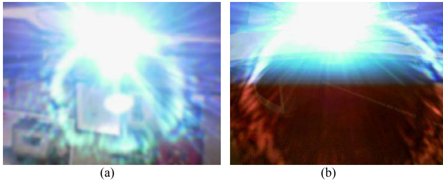
Figure 4. Images taken from a camera hit by localized light beam emitted by our camera neutralizer. The picture on the left shows a localized light beam generated using a single color. The picture on the right shows a localized light beam generated using color patterns that do not allow the cameras to adjust to the light source (notice the scan line).
