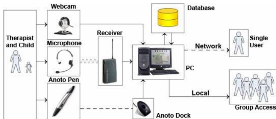
Figure 3: This shows the basic system setup to run and interact with Abaris.
